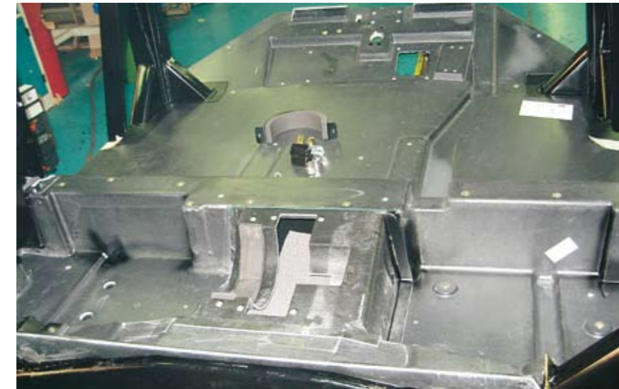
Preformed floor bonded to the steel frame
