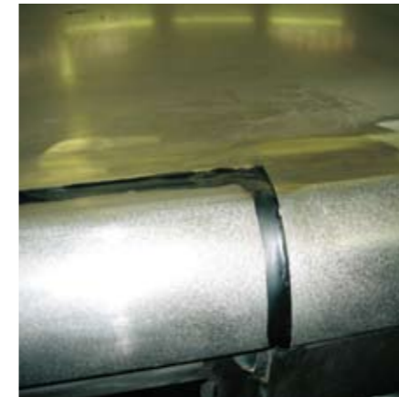
Cabin roof welded and sealed before e-coat
