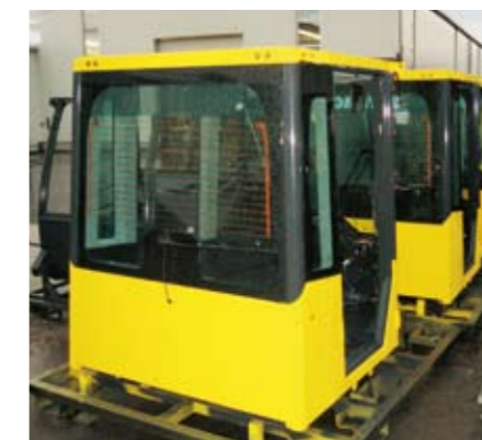
Direct glazed cabin after leakage test
