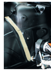
Spray seam sealing
