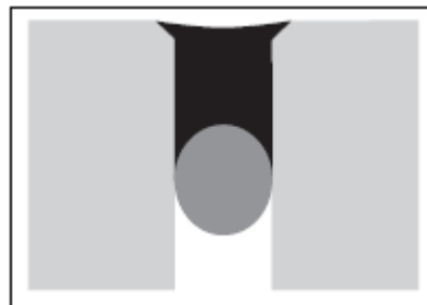
Flush joint design rules out trip hazards and dirt traps
