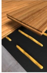
The unique and patented Sika **AcouBond System** can improve both impact sound and the ambient sound on wood floors substantially. Impact sound is reduced up to minus 18db and the wooden boards are securely fixed to the subfloor. The **Sika® AcouBond®** system is therefore an ideal combination of a floating installation and a fully bonded wood floor installation.
