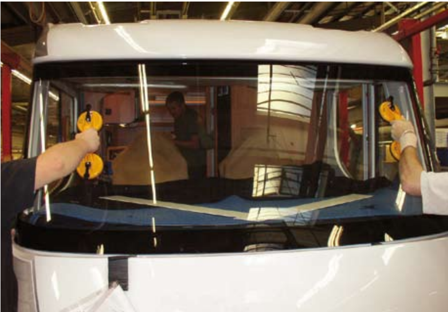
Installation of a direct glazed windshield
