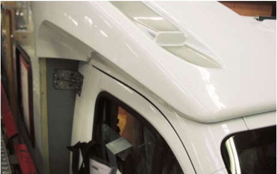
Bonded roof of a semi-integrated motorhome
