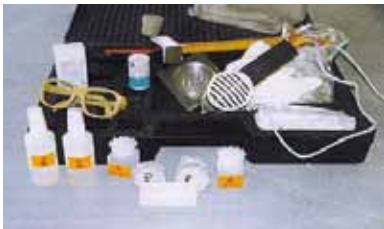
The Sika Qualitative Colour Test Kit for Penetration Depth testing
