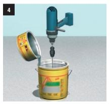
Mix **Sikadur**°-**Combiflex**° **CF** adhesive components A and B for a minimum of 3 minutes until the mix is homogeneous.
