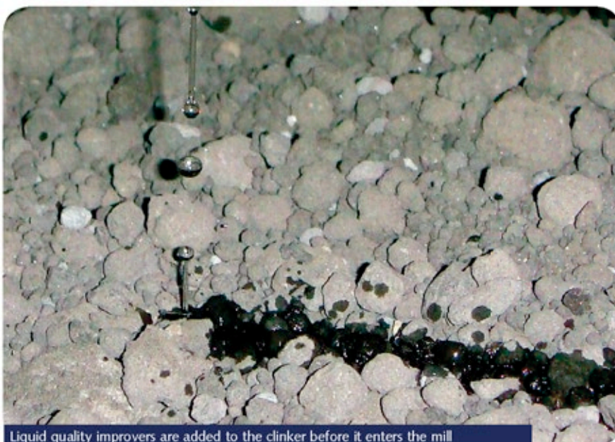
Liquid quality improvers are added to the clinker before it enters the mill
