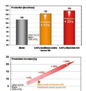
Figure 4 (right): PCE powered GA increases the production significantly.
