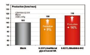
**Figure 6:** PCE powered GA increase the production significantly.
