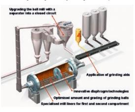
Figure 1 (right): Improvements of clinker grinding. deemed to already be at its limit. Indeed, the grinding process has been subject to a large number of improvements over the last few decades. Completely new mill systems for pre- and fine-grinding have been developed, and furthermore, the most widely spread ball mill system has seen several steps of improving its efficiency that have resulted in increased production rates and reduced specific energy consumption levels (see Figure 1).
