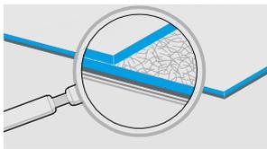
Felt as a leveling or separating layer with an adhesive layer, which enables the membrane to be fully bonded directly to the substrates. These are typically used for fast application and in adhered systems where aesthetics is a must.
