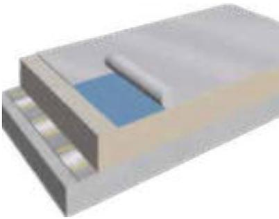
The membrane is adhered to the full surface of the substrate, giving the highest quality of aesthetic appearance. This type of application can be carried out in 2 ways:
