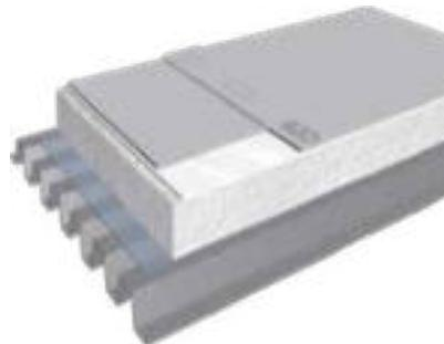
In spot fastening systems the membranes are fixed using steel screws (Sarnafast® 4.8 or 6.0 mm in diameter) with pressure plates or plastic tubes anchored into the deck.
