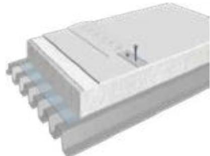
In the Sarnabar® system (fastening bars), the sheets are loose laid and secured using the fastening bars anchored to the deck. The bars are then covered with additional strips of the same membrane and welded to the waterproofing layer. This system provides high resistance to wind uplift because loads are transferred through the fastening bars to the supporting roof structure.
