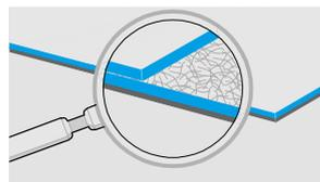
Felt as a leveling or separating layer, it provides keying for the adhesive bond. These are typically used in adhered systems or roofs where aesthetics is central.
