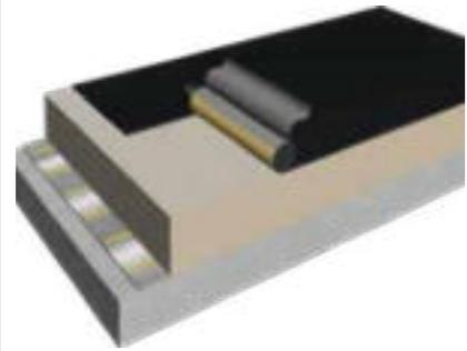
Self adhered membranes have a factory manufactured adhesive film on the back side of the membrane which is rolled out and bonded directly to the substrate when its release liner is removed.
