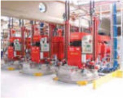
Sika's polyurethane coatings are produced using automated plants with electronically measured and dosed raw materials in stainless steel dissolving mixers. Each production unit has a powerful motor, its own heating and cooling system and an automatic discharging and cleaning system. Products are then packaged in steel drums.
