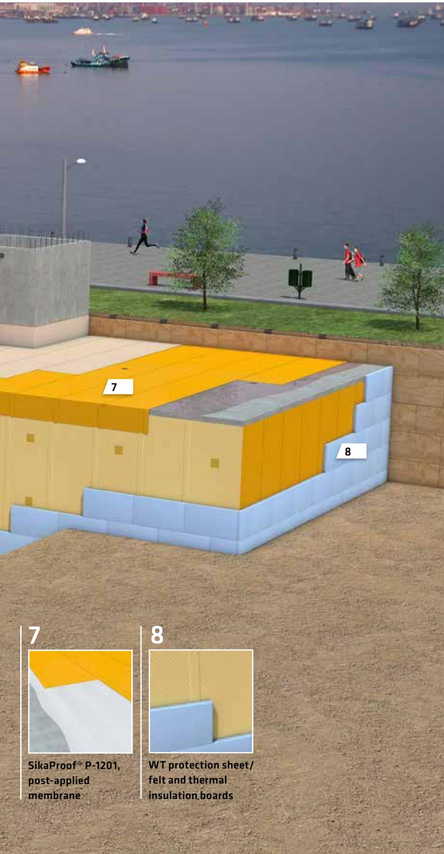
The SikaProof® system consists of two alternative methods of installation:
