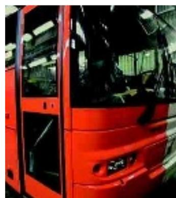
Finished glass installation including gap-filling
