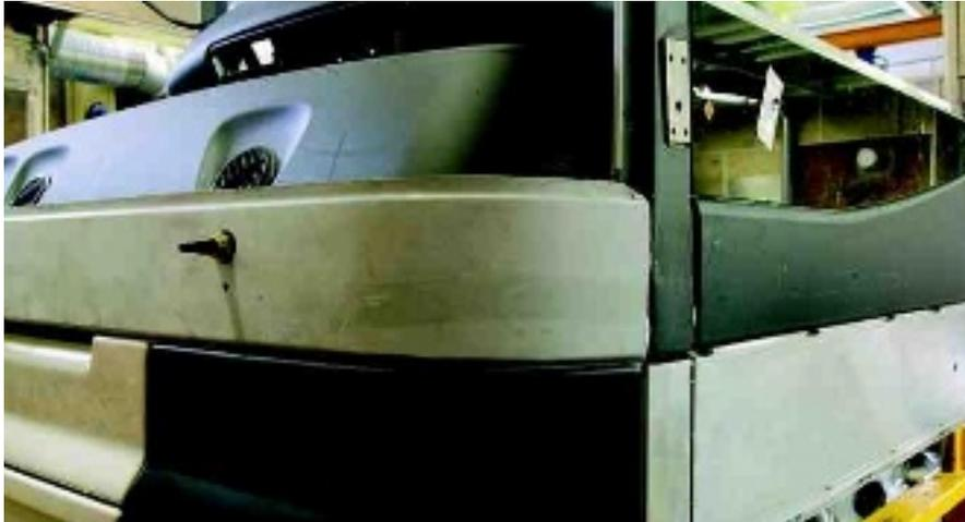
Assembly of GRP rear module onto aluminium structure
