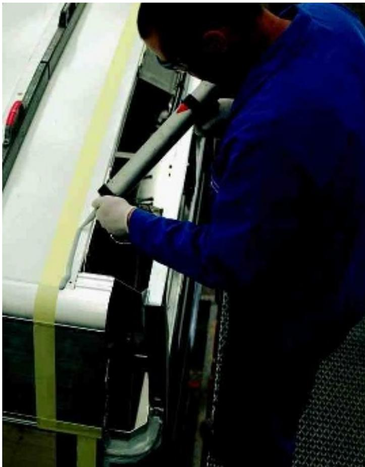
Bonding of aluminium roof onto aluminium frame
