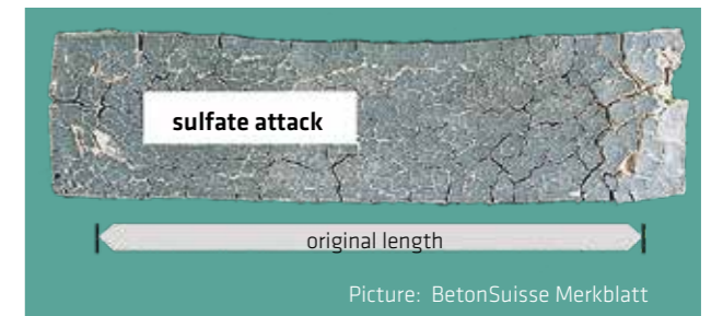
Sulfate driven attack is caused primarily by sulfates dissolved in water. By reacting with the hardened cement matrix, an increase in volume is induced which damages the structure.
