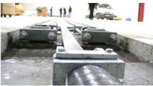
Base channel with post-tensioned CFRP plates
