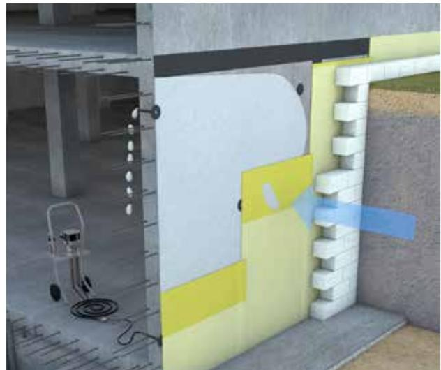
1. Remove the face-plate from the junction box and expose the Control Tube vent ends for the leaking compartment. Connect a Sikaplan® W Injection Piece to one vent end.
