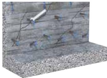
**2.** Install the mechanical packers. Tighten the mechanical packers so that they can withstand the maximum injection pressures.
