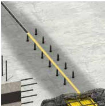
■ Waterproofing construction joints with and without hydrostatic pressure
