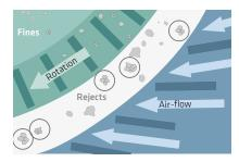
Agglomerates of sufficiently ground particles are detected by the separator as coarse particles and consequently return as reject to the mill.
