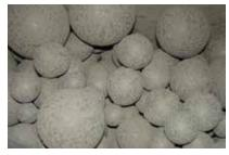
■ These attraction forces are the reason why ground particles stick on mill internals (coating effect) and soften the impact of the grinding media.
