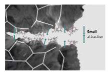
SikaGrind® ensures that the particles stay separated, thus enabling sufficiently fine particles to leave the mill and creating space for coarse particles to be refined.
