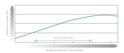
Traditional grinding aids are based on amino alcohols and glycols which can be used in formulated products, but also as pure raw materials. Sika has developed a polycarboxylate polymer powered grinding aid technology which is able to improve the performance of traditional technologies. The major benefit of this new technology can be measured in a distinct production increase which arises from an intensified particle dispersion.
