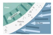
■ Particles treated with SikaGrind® are better dispersed when entering the separator. The higher the powder dispersion, the greater is the probability that the particles are detected with their actual dimension.
