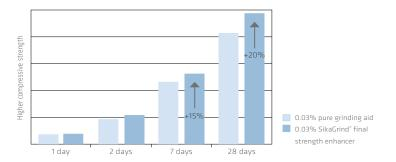
Final strength enhancement with SikaGrind® at increased production
