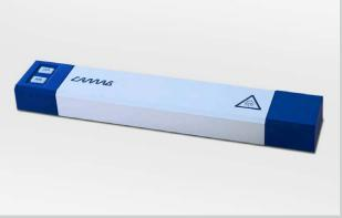
Detection by simple UV torch that provides the required wavelength of 320 nm - 420 nm.
