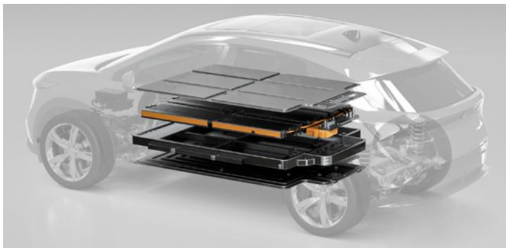
Enclosing the battery pack, also called battery lid sealing is made secure with Sikaflex® materials. After application, the wet applied product will conform to many surfaces and allow for tolerances across the pack to achieve the seal required from water, air and dust ingress. Sika can support these applications with adhesion tests to the materials used in the pack to ensure the right product is chosen for the application.
