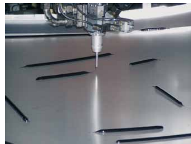
Anti-flutter bonding and sealing using SikaPower® 2C
