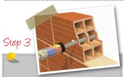
Pump approximately twice until both parts come out uniformly. Do not use this material! Inject adhesive into the perforated sleeve while slowly drawing back the static mixer. Avoid entrapping air.
