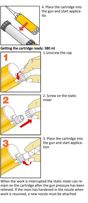
When the work is interrupted the static mixer can rerelieved. If the resin has hardened in the nozzle when work is resumed, a new nozzle must be attached.
