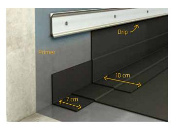
Along the perimeter of the roof and on the flat, the membrane should be bonded completely to the substrate. Same when applied with slopes higher than 15°: the membrane must be mechanically attached at the top.
