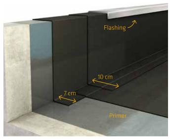
If the waterproofing membrane comes up to the top of perimeter walls, it must then be covered with a nailed flashing.
