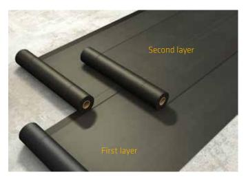
If the layers do not adhere well to each other, the water can pass through the innumerable "channels" existing. The security of a multi-layered membrane is ensured exclusively by the complete adhesion between the layers, which make it up.
