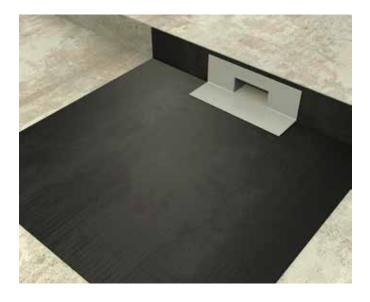
Cut and apply another piece of the membrane, enough to cover 15 cm higher than the size of the drain and more 10 cm on the top. Cut more two pieces of the membrane, enough to cover 10 cm of the top and the surface. Then apply on both sides of the drain.
