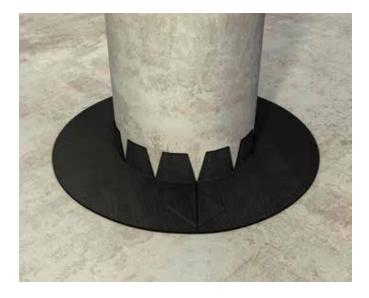
■ Cut another piece of membrane, same size as the first, and bond on the opposite direction. Then proceed with the application of the first layer of the bituminous membrane.
