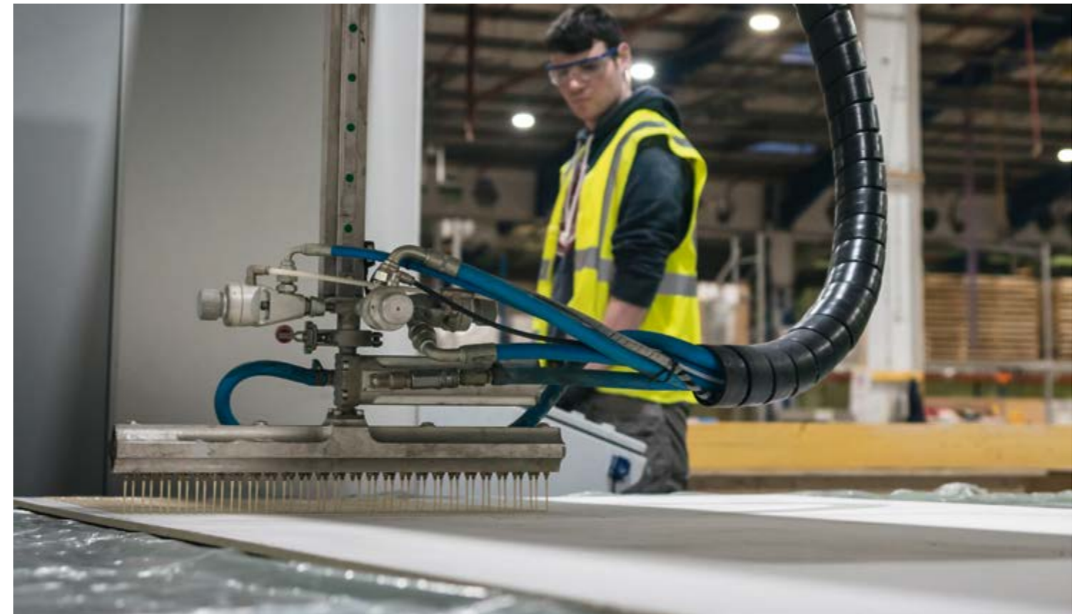
SikaForce® applied by spreader bar
