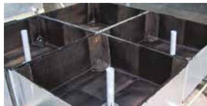
2. Test containers waterproofed with DEFEND ANTIROOT
