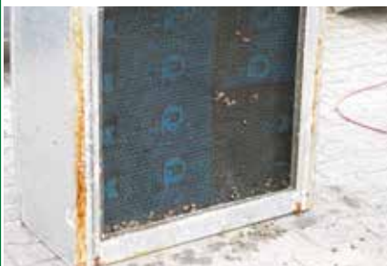
9. Unchanged under face of DEFEND ANTIROOT after the test
