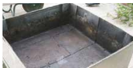
8. Unchanged upper face of DEFEND ANTIROOT after the test
