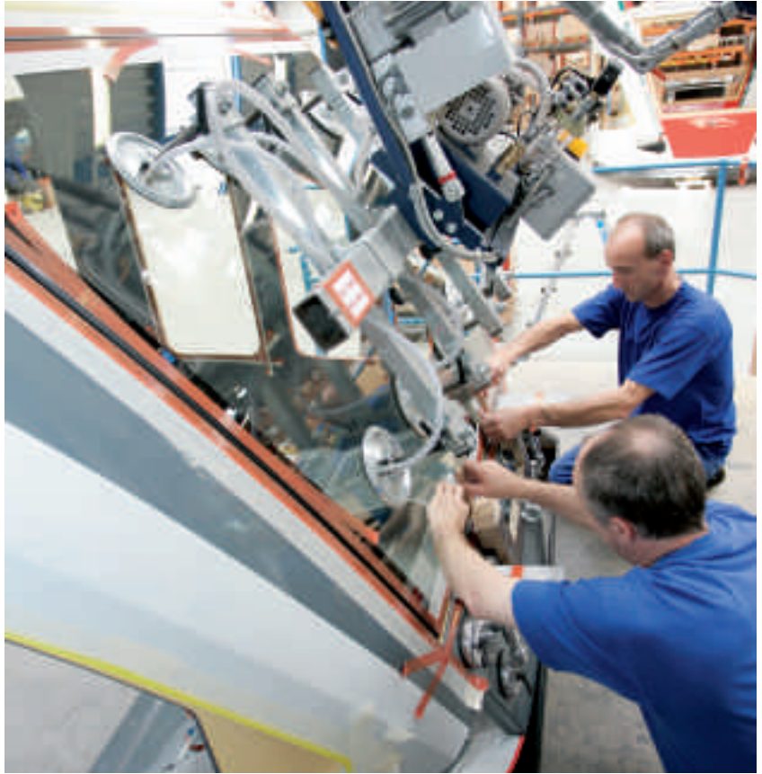
The windscreen is fitted
