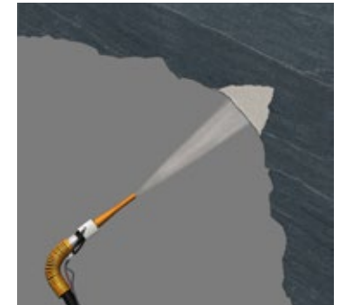
Fig. 7.2: Filling of overbreaks
