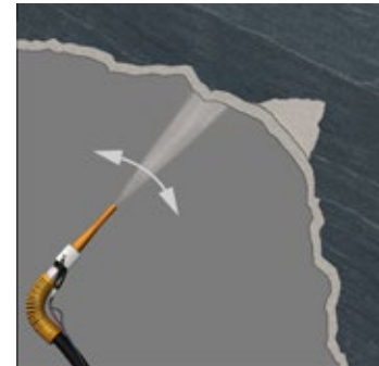
Fig. 7.3: 1st shotcrete layer – 1 st excavation stabilization and adhesive bridge for the 2 nd shotcrete layer
