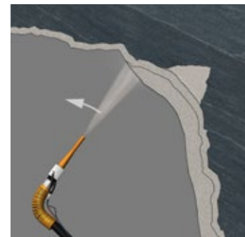
Fig. 7.5: 2 nd shotcrete layer – excavation stabilization, usually together with steel reinforcement
