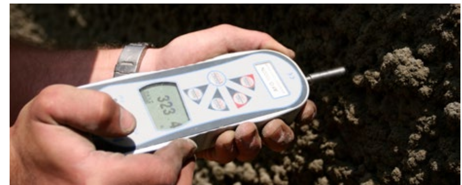
Fig. 8.3: Penetration of freshly sprayed concrete using a digital penetrometer (Mecmesin AFG 1000)
