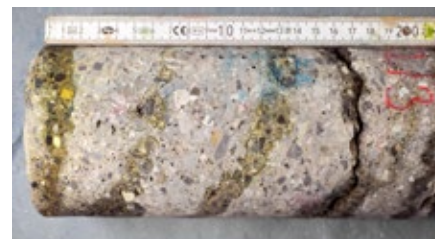
Fig. 7.13: Well visible spraying layers in a drill core
