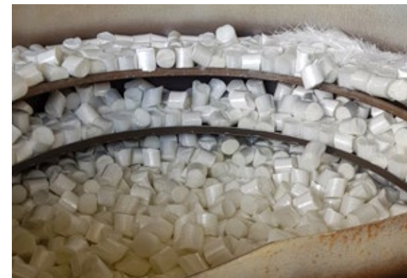
Fig. 4.8: SikaFiber® Force-60 PP fibers automatically dosed in the production of sprayed concrete as pucks wrapped in water-soluble foil.
