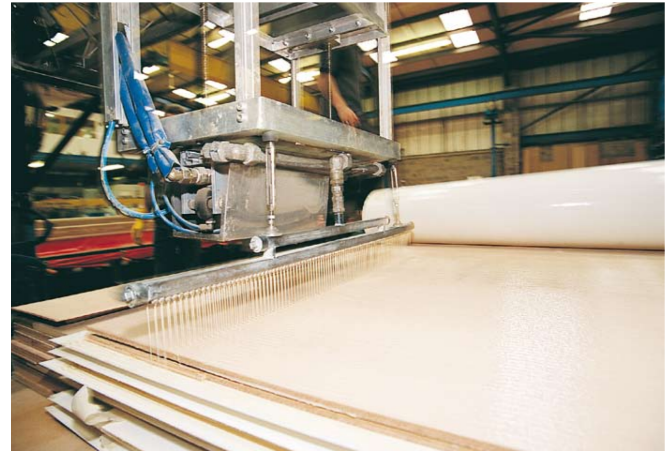
SikaForce® applied by spreader bar
