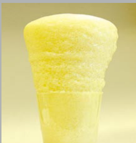
The free expansion rate of Sika® Injection-101 RC is up to 40 times.
