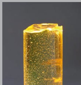
Sikadur®-52 Injection achieves a strength of up to 50 N/mm 2 .
