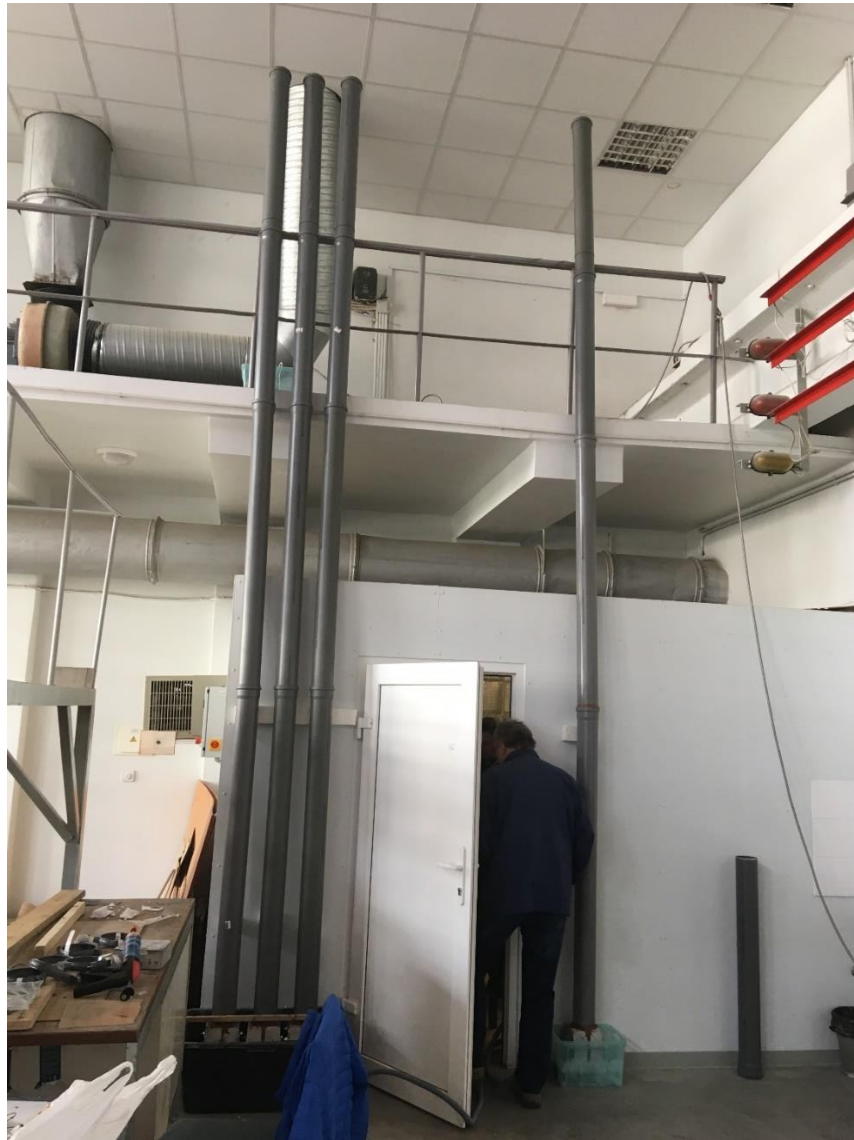
Fig. 7. Testing procedure of crack healing effect with 5-meter high water column pressure (is about 0.5 atmospheric pressure on specimen).
