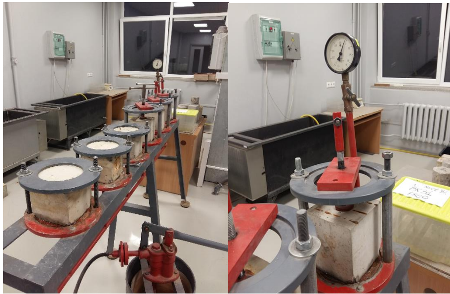
Fig. 3. Water impermeability test in special frame
