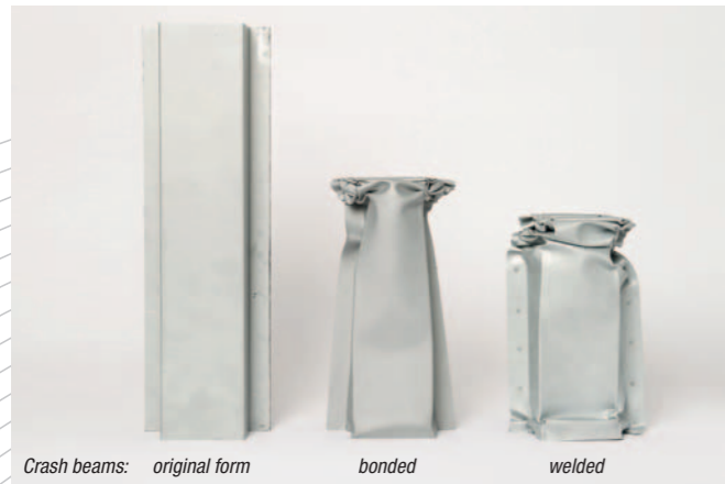
Crash beams: original form bonded welded
