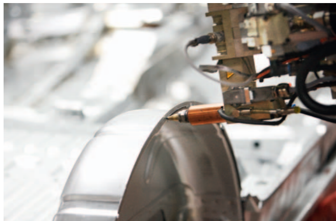
Fully automated SikaPower® wheel arch application
