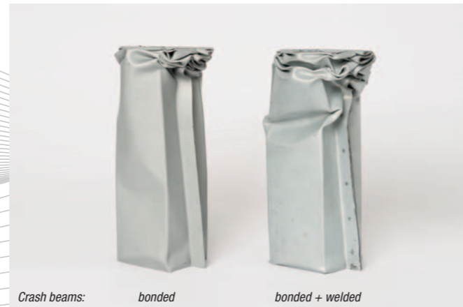
Crash beams: bonded bonded + welded
