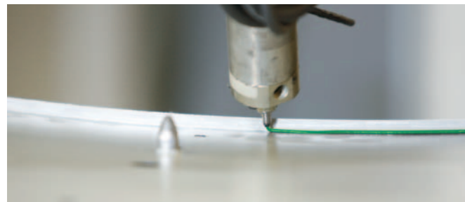
Fine jet SikaPower® hem-flange application
