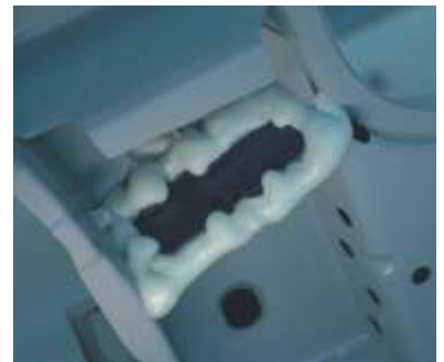
The moulded baffles turn to foam during heat treatment, adhering to the adjacent surfaces, forming an effective vibration absorbent filling
