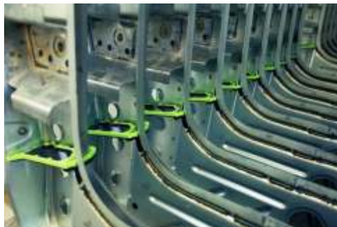
A series of moulded baffles fitted inside the frame
