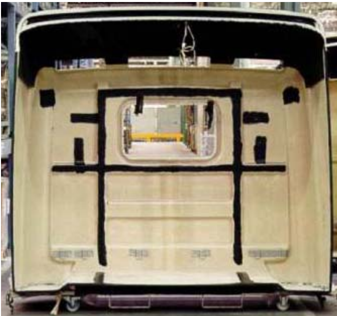
A series of high roof units waiting for assembly The units are prepared with Sika® Primer (the black areas)
