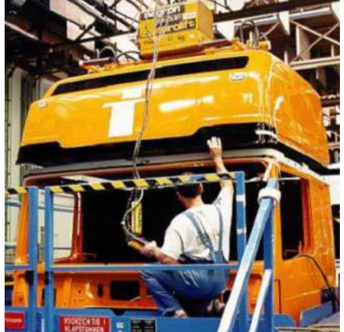
A high roof unit being fitted
