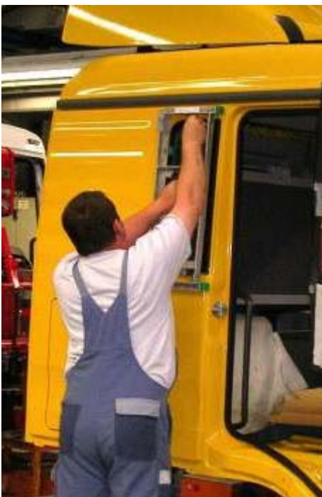
Side windows being fitted manually
