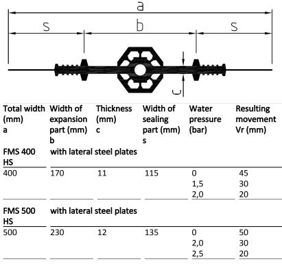
Form FM / FMS ... HS with central hose sheating are used for compression joints with shear stress or joints with a width Wnom > 30mm. Vr = Resulting movement Vr =  $(v_x^2 + v_y^2 + v_z^2) \frac{1}{2}$
